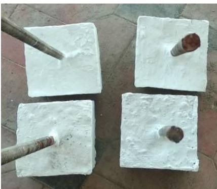
Fig. 2 Specimens for pull out test
