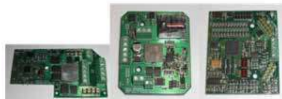
Fig 12. The Voltage Regulation Card .Middle: The battery Charge card. Right: Joint Controller card
