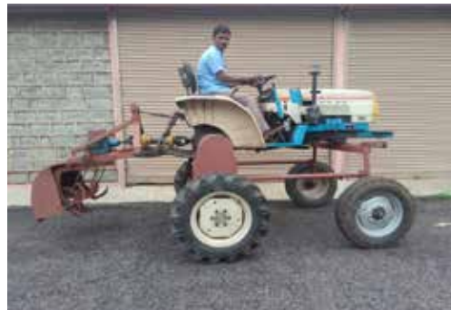
Fig. 2: High ground clearance platform for mini tractor
