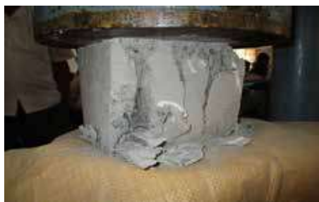
Figure 1. Testing arrangement of compression test of cube specimen
