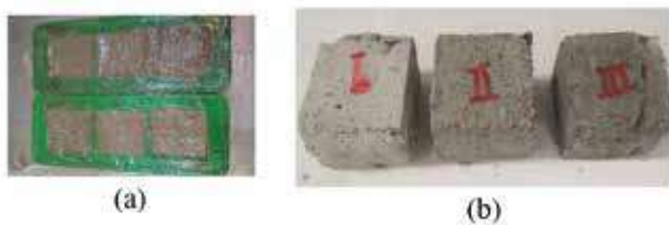
Fig. 3. (a) cube samples cast in plastic moulds, and (b) samples after demoulding, air curing and testing
