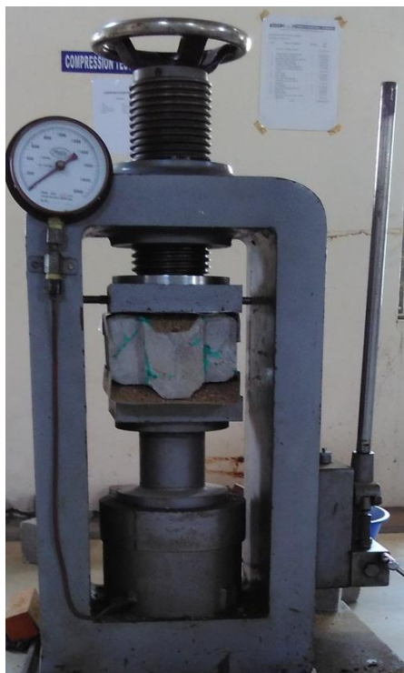
Fig-7: Compressive strength set up
