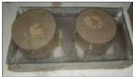
Fig. 3. Setup for sorptivity test
