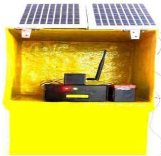
Fig. 7. ABS Chamber Compatible for Solar Mountings
