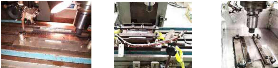
Fig. 1. Experimental setup for (a) Air cooling, (b) Forced water cooling, (c) Under water cooling
