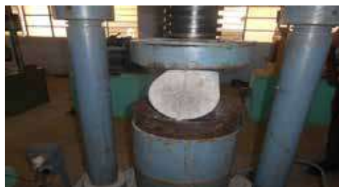
Figure 3. Testing arrangement of splitting tensile strength
