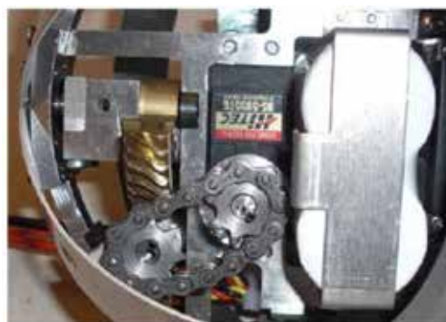
Fig 10. Roller chain connecting the servo motor to the worm gear
