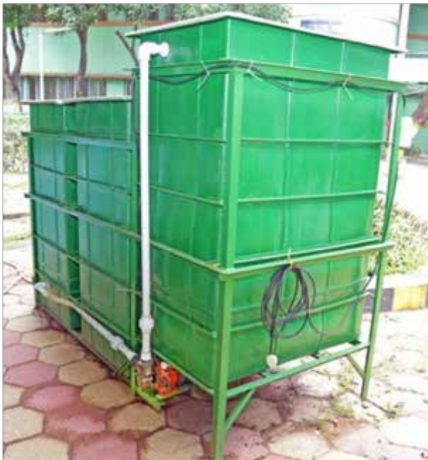
Fig. 3. Images of portable water tank for retting of jute ribbons and barky jute
