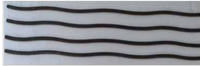
(a) typical PSWC-BARS of steel, characterized by plain surface and gentle wave-type configuration
