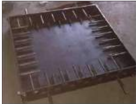
Fig. 4. Slab specimen for restrained shrinkage test
