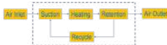
Fig. 2. Schematic of the proposed process for producing sterile air by heating method
