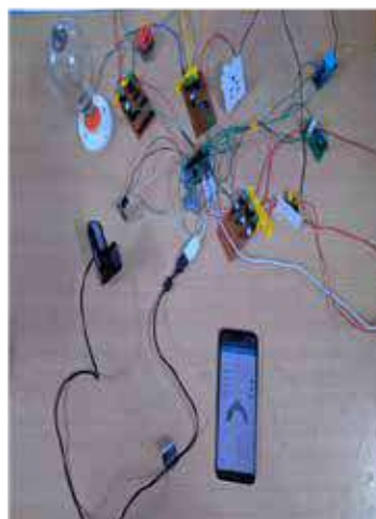
Fig. 5. Control circuit consist of Raspberry PI and relay unit.
