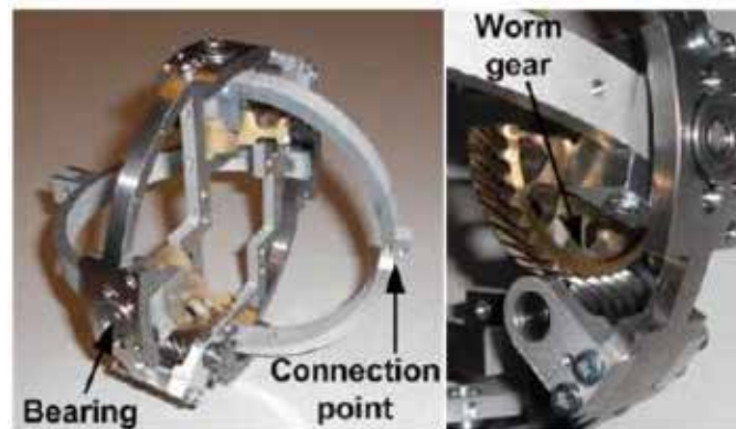
Fig 11. The articulation mechanism of the joint modules
