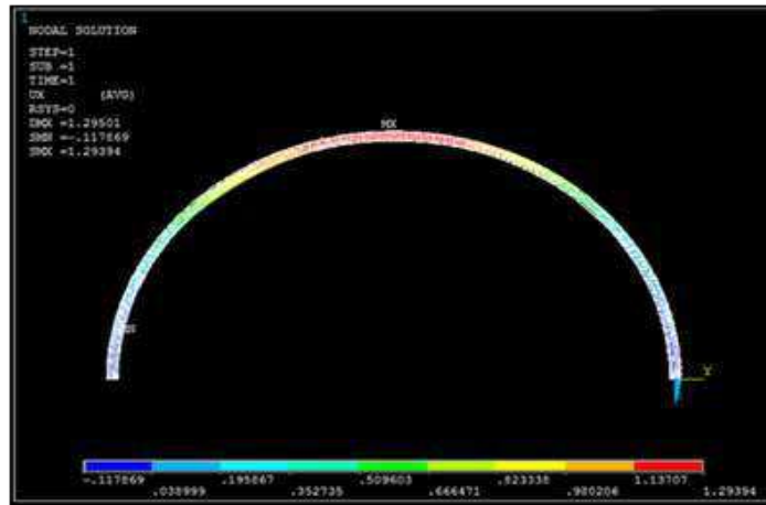
Fig. 5. Structural deformation of dia. 1m beam
