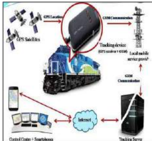
Fig. 1. Schematic of GPS / GPRS based vehicle tracking hardware
