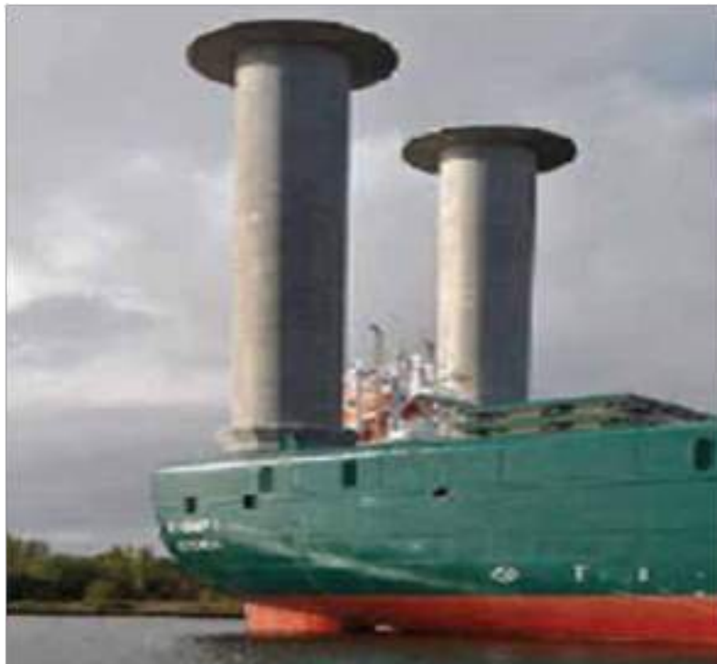
Fig. 3. Rotor sails, Flettner rotors are being developed. These utilize a so-called “Magnus Effect” for generating energy
