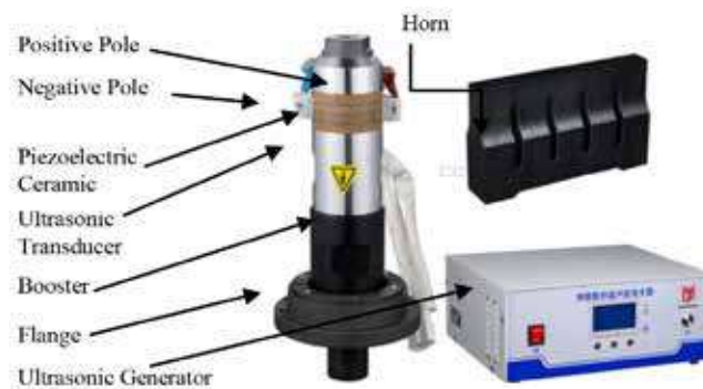
Fig. 2. Various parts of ultrasonic welding [10]
