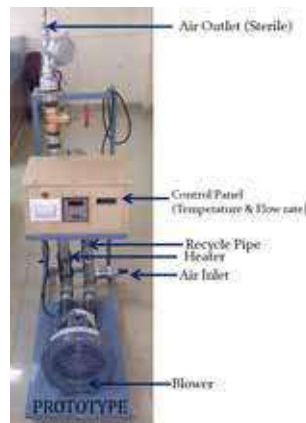
Fig. 3. Prototype of the air sterilizer developed
