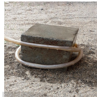
Fig. 2 The concrete cube enclosed with drip pipes.
