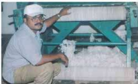
Fig. 1. Gin rollers of double roller gin are made of rubberized cotton fabric roller covering material; green design-cast study-DPR-1
