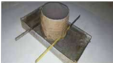
Fig 1. Experimental setup for water absorption test on super absorbent polymer
