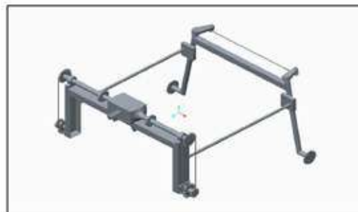
Fig. 1: CAD model of high ground clearance platform for mini tractor
