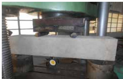
Figure 5. Testing arrangement of prism flexural strength
