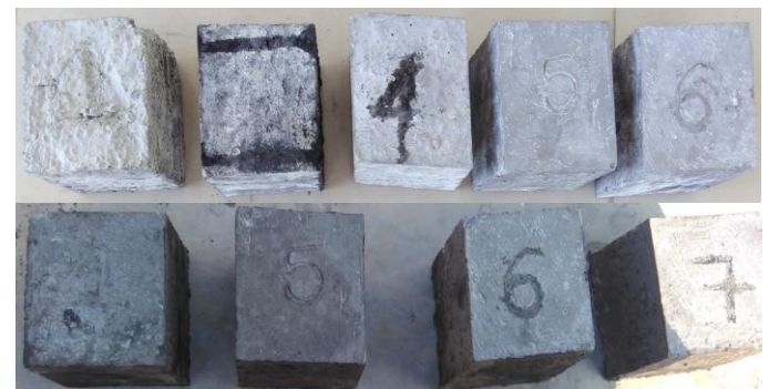
Fig -4: Cast cubes by replacement of M sand by roof tile waste in 0,5,10,15,20,25 and 30%
